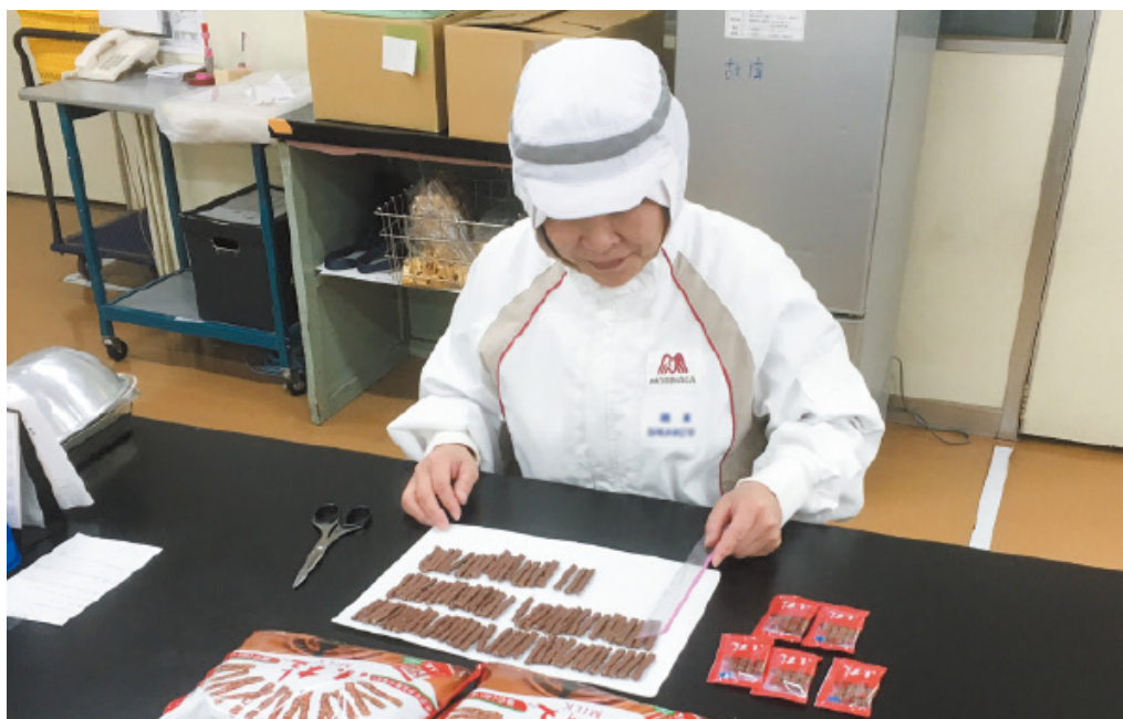
Product inspection (measurement of the length and weight to determine the adherence to specifications)
